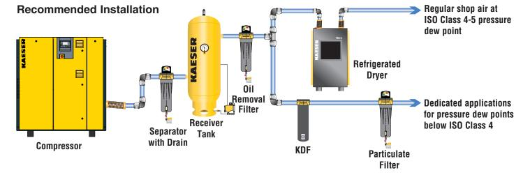
The KDF should be installed after a receiver tank. The KOR prefilter is required to protect the KDF from bulk liquid and contaminants increasing the life of the dryer's desiccant bed.
