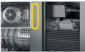
**External grease fitting lubrication**
