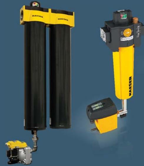
All desiccant dryers require proper filtration. Coalescing pre-filters prevent contamination of desiccant beds by hydrophobic aerosols. Particulate after-filters collect traces of desiccant dust that may exit the dryer. Maintaining these filters extends service intervals and provides excellent air quality. All Kaeser desiccant dryers offer optional filter packages with or without block and bypass valves.
