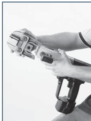
Place the jaws in the housing
