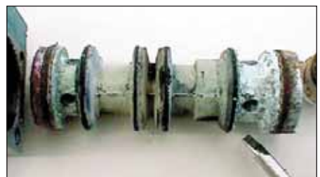
Contaminants corrode and damage air-operated equipment
